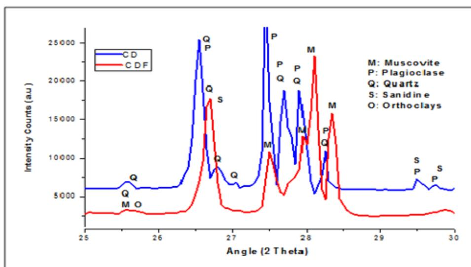
Figure 1: XRD pattern of crusher dust and crusher dust fertilizer
