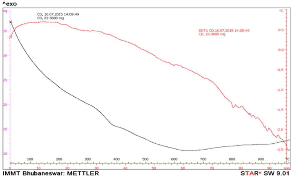
Figure 2(a): Thermo gravimetric analysis of crusher dust
